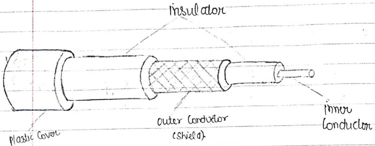
→ Coaxial cables are commonly used in telephone networks, for cable TV and radio transmissions.
