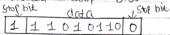
→ Addition of start and stop bits increase the number of bits.
